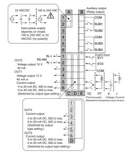
The power supply voltage must be 100 to 240 VAC or 24 VAC/DC for the E5ER-T to comply with CE <u>∧</u> Note marking requirements. The power supply voltage must be 100 to 120 VAC or 24 VAC/DC for the E5ER-T to comply with UL requirements.
