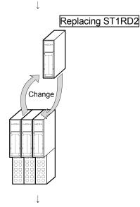
5) Remove the ST1RD2 and replace with new one.
