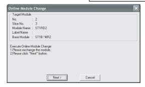
4) As the left screen appears, power off the external device connected with the ST1RD2 to be removed.
