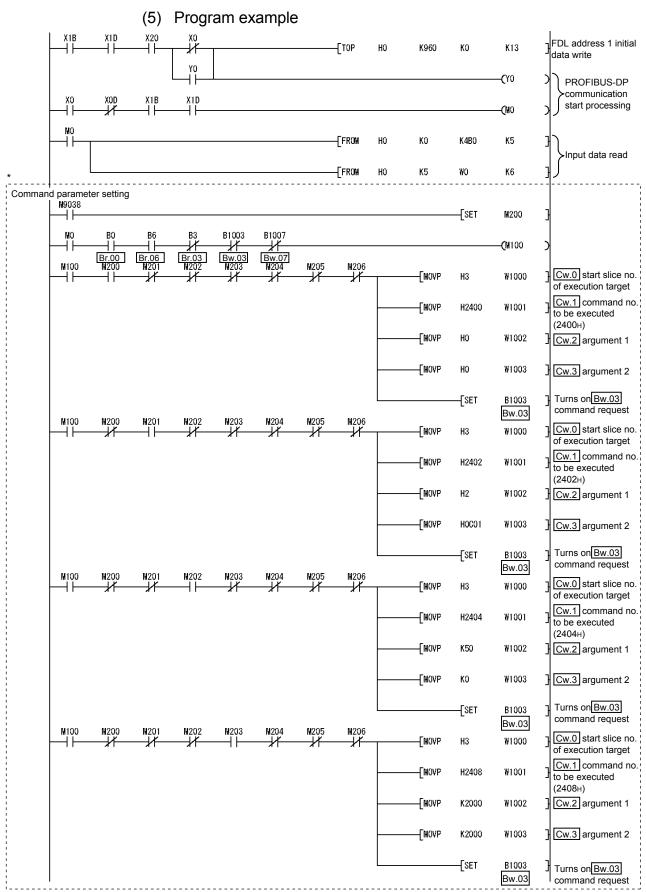
\* The program area enclosed by the dotted line is not required when GX Configurator-ST is used to set the command parameters.
