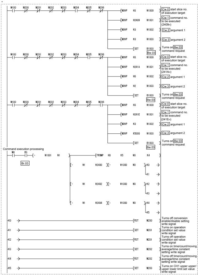
\*The program area enclosed by the dotted line is not required when GX Configurator-ST is used to set the command parameters.
