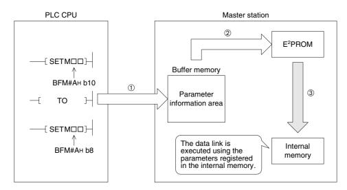
7) Data link status setting for a case where an error occurs in the CPU in the master station (PLC)
