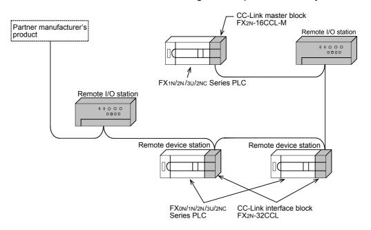
Master station : Station which controls the data link system
