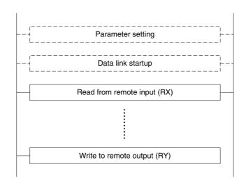
3) Create such a program that read of received data and write of transmission data are executed after the host station becomes the data link status (after the BFM#AH b1 turns ON).
