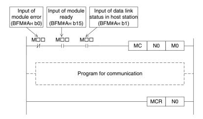
4) Create such a program that detects the data link status in remote I/O stations and remote device stations and executes interlock. Create a program for error handling.
