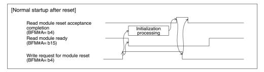
b) When the write request for module reset (BFM#AH b4) is set to ON, the read module ready (BFM#AH b15) turns OFF and the initialization processing is executed. When the initialization processing is abnormally completed, the read module ready (BFM#AH b15) does not turn ON, but the read module error (BFM#AH b0) turns ON instead.
