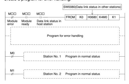
5) The auxiliary relays in the non-keep area (example: relays marked with "O") must be used as auxiliary relays (M) for parameter setting programs.
