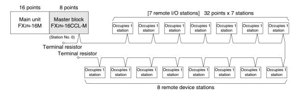
In the FX2N Series PLC, when a 16-point basic module and the master block FX2N-16CCL-M are connected, up to 7 remote I/O stations can be connected (7 is the maximum number). As to remote device stations, up to 8 stations can be connected without regard to the number of remote I/O stations.
