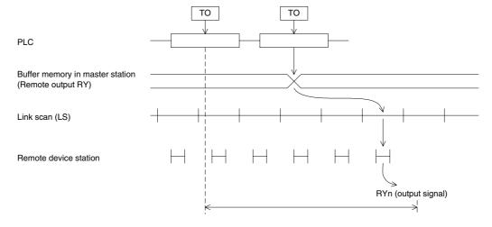
3) Master station (RWw) → remote device station (RWw)
