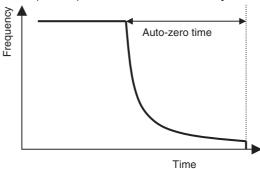
When there is no input pulse for a specified time, auto-zeroing can be used to force the measurement frequency to zero. The time from cutoff of the input pulse to the zeroing of the measurement frequency is called the "auto-zero time."
