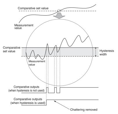
Hysteresis works in the direction of decreasing measurement values for comparative set values HH and H and works in the direction of increasing measurement values for comparative set values LL and L. Note that hysteresis works in the direction of decreasing measurement values for all set values if the output pattern is set to a level output.
