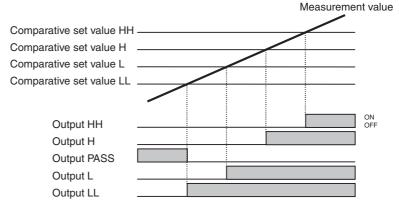
\* The PASS output turns ON when any of the HH, H, L, and LL outputs turns OFF.
