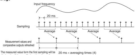
The measured value form the first sampling will be displayed until the specified number of samplings is performed up to the first averaging time.  $20 \text{ ms} \times \text{averaging times}$  = 80 ms
