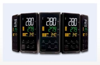
A wide viewing angle was achieved with the LCDs to enable easy confirmation of the PV.
