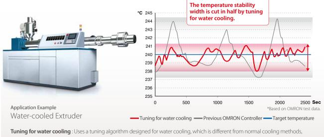
to automatically set the optimum PID constants for water cooling.
