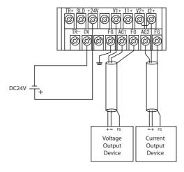
$Ch\ 1\ output\ voltage\ terminals ... V1+,\ AG1,\ FG$   $Ch\ 1\ output\ current\ terminals ... I1+,\ AG1,\ FG,\ V1+$   $Ch\ 2\ output\ voltage\ terminals ... V2+,\ AG2,\ FG$   $Ch\ 2\ output\ current\ terminals ... I2+,\ AG2,\ FG,\ V2+$   $When\ inputting\ current,\ be\ sure\ to\ short\ I^*+\ and\ V^*+.$
